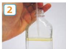
oils will be extracted by the solvent and transferred to a cuvette
