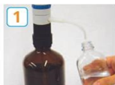
Add the solvent to the water sample to be analyzed and shake
