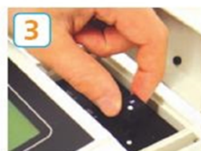
Place the cuvette into the instrument and the reading will be displayed
