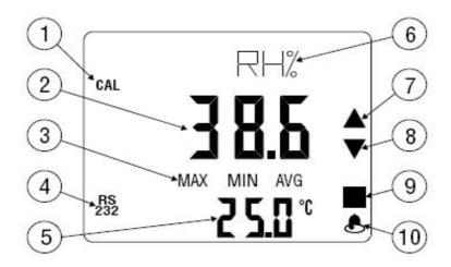
The display constantly shows the measure of two quantities. In line 2 the size can be selected by pressing MEAS, in line 5 at the bottom is always displayed temperature. During measurement, the top line 6 displays the unit of measurement of the main variable; the menu provides information on the active voice.
