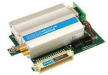
**Network Interface:** mobile telephony to access the internet through GSM & 3G networks.
