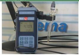
PH105.1 without datalogger function but with an RS232C serial port for real time transfer of acquired measurements. PH105.2 full version, with RS232C serial port plus datalogger function up to 34,000 pH and temperature reading, configurabled by user menu, which can be transferred to a PC by multi-standard RS232C serial port or USB 2.0. Storing interval, printing, and baud rate can be configured by menu.
