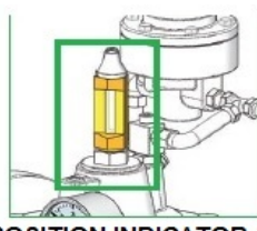
POSITION INDICATOR AND RELIEF VALVE
